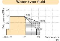
A rough guide to the service life of this gasket when it is used as a pipe gasket to seal steam of 100°C or higher is as follows.
