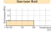
Do not use TOMBO  $^{\text{TM}}$  No.1993 for gas type fluids where even minute amounts of leakage are not allowed. Even for use with the water- or oil-type fluid, be sure to use paste when carrying out an airtightness test. It is recommended to use TOMBO  $^{\text{TM}}$  No.1133 or TOMBO  $^{\text{TM}}$  No.1120 instead.
